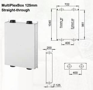
Standard 4x 125mm Ports are placed at the top and bottom of the item to give straight through duct connections. Compact design with easy installation and maintenance. Please see above image for the individual dimensions. Unit supplied with two inspection covers, one on each side enabling the unit to be left or right handed.
