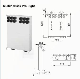
The standard 2x6 Supply and Extract Airflex Pro connections are orientated 90 degrees to the main body. 1x extra port for supply and extract is located on the side of the unit. These are facilitated by knockout points. Compact design with easy installation and maintenance. Please see above image for the individual dimensions. The supply air to the dwelling is on the right hand side in this unit as you look at the unit.
