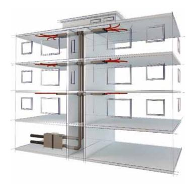
The MultiPlexBox is a great air distribution unit for blocks of flats or apartment buildings. In just one compact unit, the MultiPlexBox perfectly combines the following four features: volume flow control, virtually silent operation, efficient air distribution and demand-driven control.
