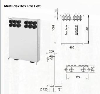
The standard 2x6 Supply and Extract Airflex Pro connections are orientated 90 degrees to the main body. 1x extra port for supply and extract is located on the side of the unit. These are facilitated by knockout points. Compact design with easy installation and maintenance. Please see above image for the individual dimensions. The supply air to the dwelling is on the left hand side in this unit as you look at the unit.
