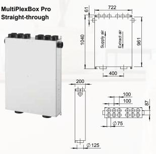
The standard 2x6 sets of Supply and Extract Airflex Pro connections are orientated to give straight through duct connections. 1x extra port for supply and extract is located on the side of the unit. These are facilitated by knockout points. Compact design with easy installation and maintenance. Please see above image for the individual dimensions. Unit supplied with two inspection covers, one on each side enabling the unit to be left or right handed.
